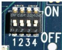
Control4 recommends you remove power from the unit prior to making DIP switch setting changes. However, if this scenario isn't an option, the installer needs to know that DIP switch changes will cause the product to reset, similar to how the device responds when turned on initially. This response is normal operation.
